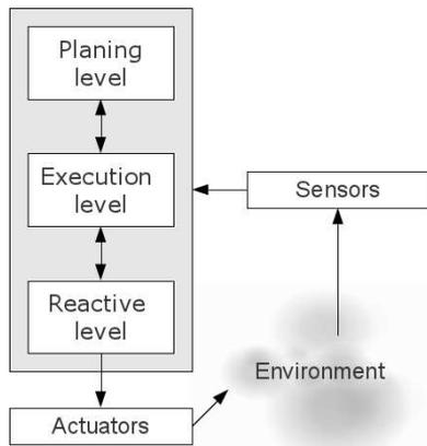
**Fig.5. Robot guide software architecture.**
