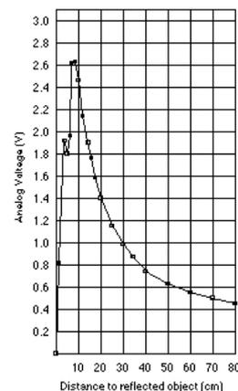
**Fig.8. Nonlinear characteristics obtained from infrared rangefinders.**
