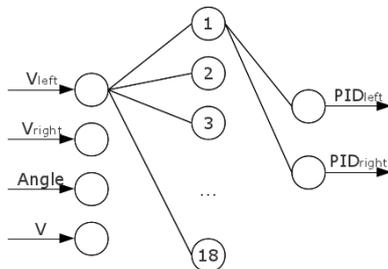
Fig 10. Architecture of PID regulator neural network.
