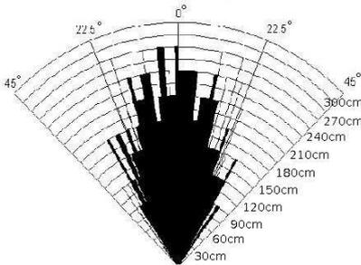
Fig.9. Directional diagram for Seedstudio Ultrasonic range measurement module.
