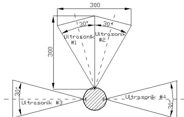
**Fig.4. Ultrasonic sensor model.**
